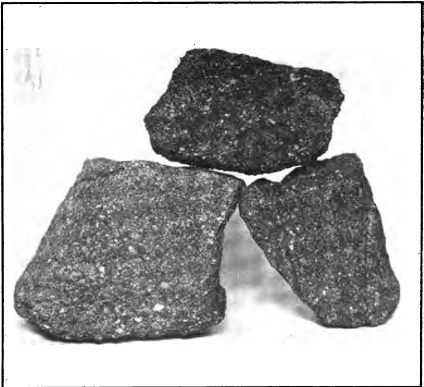
PLATE XIII(b).—Squaw Sand taken from Chloe Copenhaver well No. 2, Blue Creek Oil Field, one-half size.
